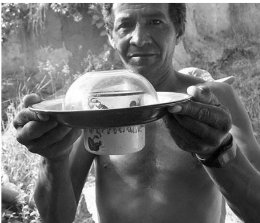
A Kitchen Bowl Retort in Brazil. The bowl traps mercury vapor during the roasting process. The mercury can be collected and reused.
